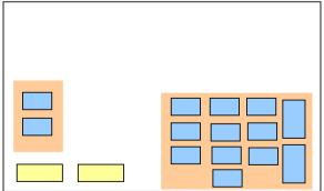
**Example 3** – this screen uses Mouse and XFS Data modes – Mouse mode is used only in a restricted area. The touch keyboard definition has 3 frames. Frame 1 has no Touch Keys. Frame 2 has 2 Touch Keys; Frame 3 has 12 Touch Keys.
