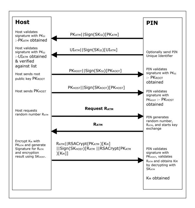
This following is a typical interaction for the exchange of the initial symmetric master key when the PIN device and Service Provider supports the Enhanced Signature Remote Key Loading scheme.
